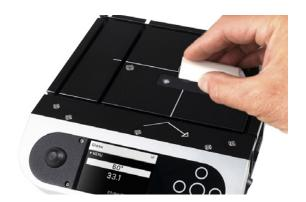
**STEP 2:** Using the continuous read setting on the Novo-Curve the sample areas were measured and the maximum values recorded for each area.
