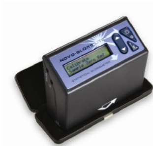
Place the instrument in the calibration holder.
