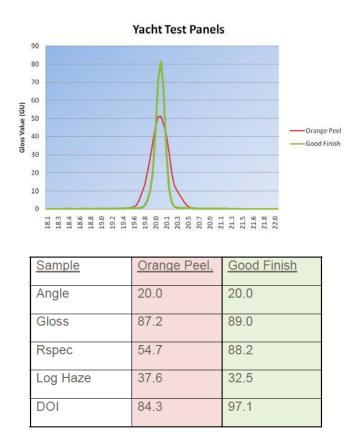
This example perfectly demonstrates the need for additional appearance information than that supplied with a glossmeter, as the panels have virtually identical gloss when measured with this instrument. Visual inspection however, shows that the first panel has a very high degree of orange peel.
