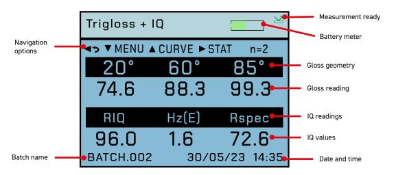
With the unit switched on and initialised the IQ will display the Home screen as shown below.
