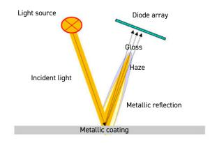
The Rhopoint IQ captures compensation information from a region adjacent to the haze measurement angle, this means it can be used on metallic coatings which reflect ligh directionally
